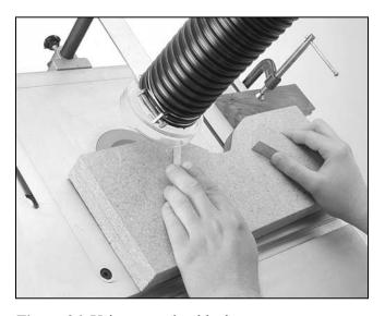
Figure 26. Using a starting block.
